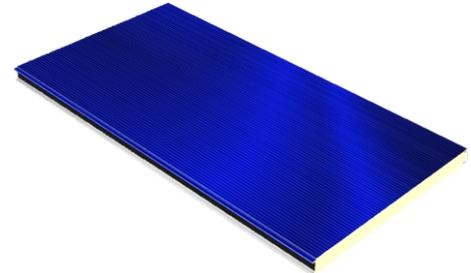
'POLAR' thermal insulation wall panel, with a visible fastening system, with (upper and lower) sides made of (PES, PVDF..) galvanised steel sheets with galvanic protection, and with a 80 mm thick expanded polyurethane core.
